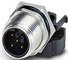
Sensor/actuator flush-type plug, 5-pos., M12, shielded, B-coded, rear/screw mounting with M12 thread, with straight solder connection
