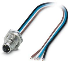
Device connector rear mounting, Power, 4-position, Pin, straight, M12-Standard, L-coding, on free cable end, Individual wires, cable length: 0.2 m, 2.50 mm<sup>2</sup>, PEX litz wire, potted, this item is expected to be lead-free from Q1 2026 in accordance with RoHS II without exception 6c (Pb < 0.1%), a lead-free alternative is possible on request in advance
