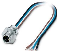
Device connector front mounting, Power, 4-position, Pin, straight, M12-Standard, L-coding, on free cable end, Individual wires, cable length: 0.2 m, 2.50 mm<sup>2</sup>, PEX litz wire, potted, this item is expected to be lead-free from Q1 2027 in accordance with RoHS II without exception 6c (Pb < 0.1%), a lead-free alternative is possible on request in advance
