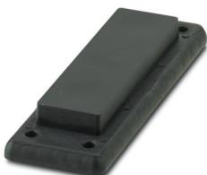
Cable feed-through plates, no. of conductors: 10, external cable diameter: 6x 2 mm ... 8 mm, 2x 2 mm ... 18 mm, 2x 2 mm ... 30 mm, material: PP (Core), material: TPE-SEBS (external material), color: black, length: 154 mm, width: 56 mm, height: 20 mm
