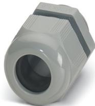
Cable gland, material for screw connection: PA, application: Standard, external cable diameter 4 mm ... 8 mm, shielding: no, connecting thread: M16 x 1.5, color: silver-gray RAL 7001
