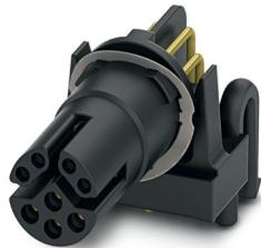
Contact carrier CAT5 (IEC 11801:2002), 8-position, Socket, angled, M12, Y-coding, Wave soldering, this item is expected to be lead-free from Q4 2026 in accordance with RoHS II without exception 6c (Pb < 0.1%), a lead-free alternative is possible on request in advance
