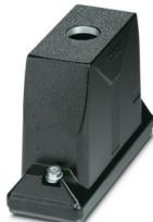
Sleeve housing B24, with screw locking, material: Die-cast aluminum, salt water resistant, cable outlets: 1, straight, 1x M25, height: 93.7 mm, cable gland: none, increased environmental requirements
