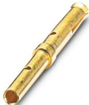
D-SUB crimp contact, Socket, turned, rated current: 3 A, connection cross section: 0.08 mm<sup>2</sup> ... 0.34 mm<sup>2</sup>, AWG 28...22, contact material: Metal
