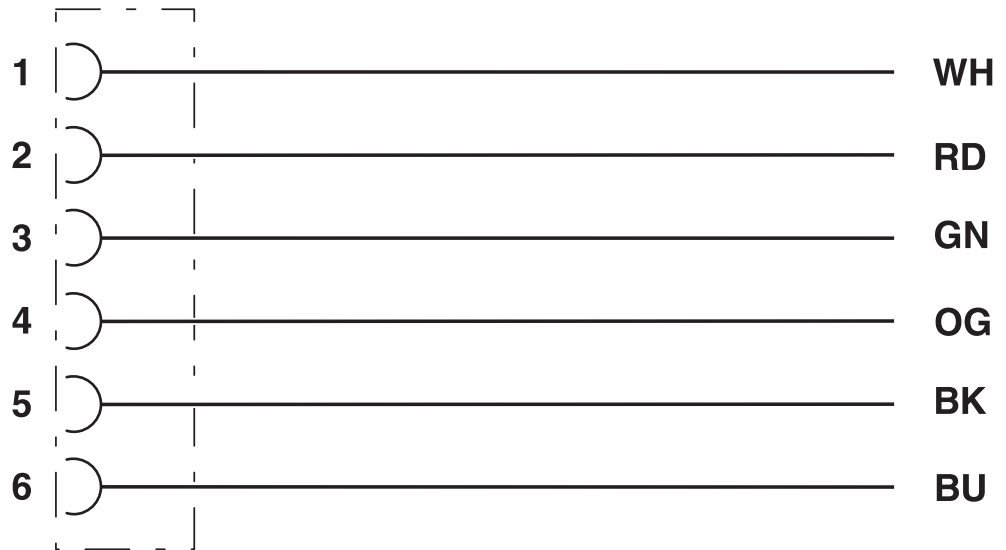
Contact assignment of 7/8" socket
