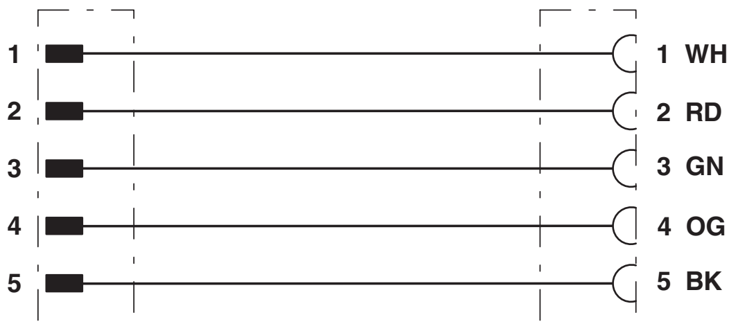
Contact assignment of 7/8" plugs/sockets
