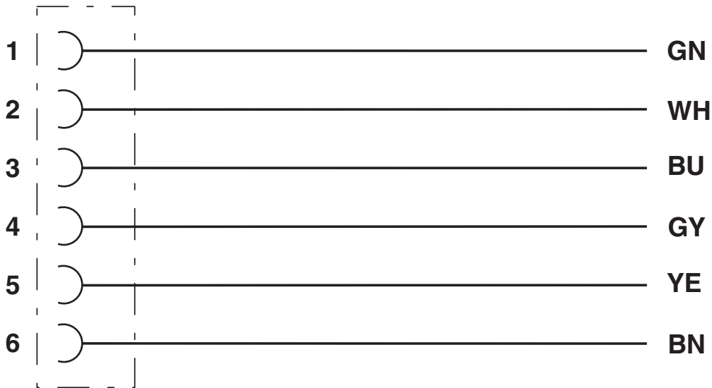
Contact assignment of 7/8" socket
