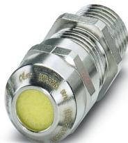
Cable gland, material for screw connection: Brass, nickel-plated, application: Ex, external cable diameter 5 mm ... 10 mm, shielding: yes, connecting thread: M16 x 1.5, color: silver-colored, with O-ring
