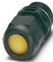
Cable gland, material for screw connection: PA, application: Ex, external cable diameter 13 mm . . . 21 mm, shielding: no, connecting thread: M32 x 1.5, color: jet black, with flat gasket
