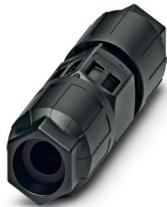
Conductor connector, connection method: IDC connection, number of positions: 2+PE, 0.5 mm<sup>2</sup> ... 1.5 mm<sup>2</sup>, 690 V, 17.5 A, PA, black, With two QUICKON nuts, coding: Coding profile, external cable diameter: 10 mm ... 13 mm
