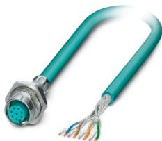
Device connector rear mounting, degree of protection: IP65/IP67, cable length: 2 m, number of positions: 8, connection method: Cable connection, Ethernet, this item is expected to be lead-free from Q1 2027 in accordance with RoHS II without exception 6c (Pb < 0.1%), a lead-free alternative is possible on request in advance, 4x2xAWG26/19, S/UTP, water blue RAL 5021
