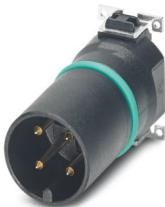
Contact carrier, 4-position, Pin, straight, M12, A-coding, SMD reflow, this item is expected to be lead-free from Q1 2027 in accordance with RoHS II without exception 6c (Pb < 0.1%), a lead-free alternative is possible on request in advance
