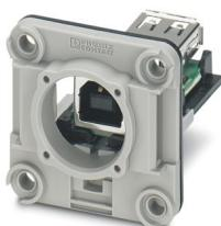
USB socket insert, 4-pos., USB socket type A to USB socket type B, socket type B to panel mounting frame side, for the Freenet system in the panel mounting frame, IP20 terminal outlet, 19" patch panel, and service interface
