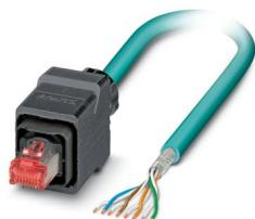
Assembled Ethernet cable, shielded, 4-pair, AWG 26 stranded (7-wire), RAL 5021 (sea blue), RJ45 connector/IP67 push/pull plastic housing to free cable end, line, length 5 m
