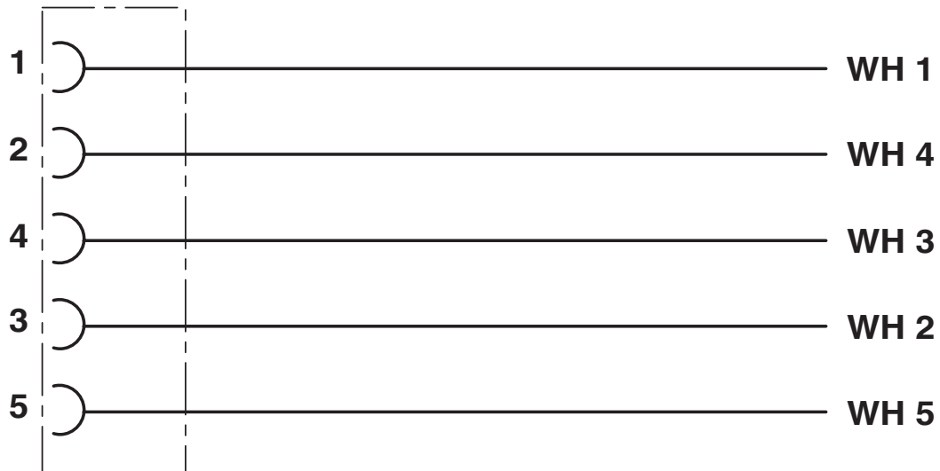
Contact assignment of the M12 socket
