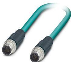
Assembled Ethernet cable, shielded, 4-pair, 26 AWG stranded (7-wire), RAL 5021 (water blue), M12 plug to M12 plug, line, length: 8 m
