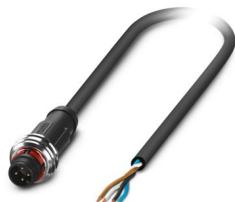
Sensor/actuator cable, 4-position, PUR halogen-free, black-gray RAL 7021, Plug straight M12 Push Pull, coding: A, on free cable end, cable length: 5 m
