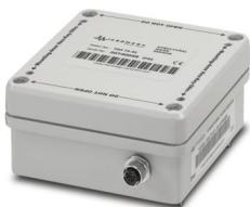
SNS 74-S1 sensor from Micromega Dynamics for detecting vibrations, damage, and imbalances on the rotor blade of wind turbine generators. Dual-axis accelerometer with temperature measurement. The measured values are available as 4 – 20 mA signals.
