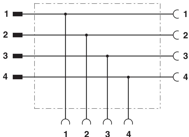
Contact assignment of the 7/8" T-distributor
