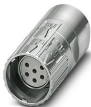
M23, Cable connector, series: M23 PRO, straight, shielded: yes, ONECLICK fast locking system, No. of pos.: 6, Direction of rotation: Standard, contact connection type: Socket, Solder connection, cable diameter range: 3 mm ... 15 mm, coding: N, Item is lead-free in accordance with RoHS II without Exemption 6c (Pb < 0.1 %)
