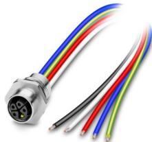
Device connector front mounting, Power, 5-position, Flush-type female connector, straight, M12-Standard, K-coding, on free cable end, Individual wires, cable length: 1 m, 2.50 mm<sup>2</sup>, PEX litz wire
