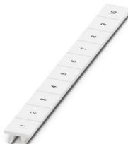
Zack marker strip, Strip, white, labeled, can be labeled with: CMS-P1-PLOTTER, printed horizontally: consecutive numbers 1 ... 10, 11 ... 20, etc. up to 91 ... 100, mounting type: latching, for terminal block width: 10.2 mm, Number of individual labels: 10, text field height: 10.5 mm, text field width: 10.15 mm
