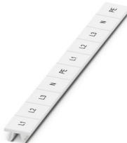
Marker for terminal blocks, Strip, white, labeled, can be labeled with: CMS-P1-PLOTTER, horizontal: L1, L2, L3, N, PE, L1, L2, L3, N, PE, mounting type: latching, for terminal block width: 10.2 mm, Number of individual labels: 10, text field height: 10.5 mm, text field width: 10.15 mm
