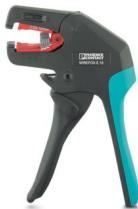
Stripping tool, for cables and conductors from 4 - 16 mm<sup>2</sup>, self-adjusting, stripping length of up to 18 mm, cutting capacity of up to 10 mm<sup>2</sup> stranded/1.5 mm<sup>2</sup> solid, replaceable stripping blade
