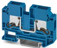
Feed-through terminal block, nom. voltage: 1000 V, nominal current: 57 A, number of connections: 2, number of positions: 1, connection method: Push-X-connection, Rated cross section: 10 mm<sup>2</sup>, cross section: 1.5 mm<sup>2</sup> - 16 mm<sup>2</sup>, mounting type: NS 35/7,5, NS 35/15, color: blue
