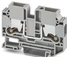
Feed-through terminal block, nom. voltage: 1000 V, nominal current: 57 A, number of connections: 2, number of positions: 1, connection method: Push-X-connection, Rated cross section: 10 mm<sup>2</sup>, cross section: 1.5 mm<sup>2</sup> - 16 mm<sup>2</sup>, mounting type: NS 35/7,5, NS 35/15, color: gray
