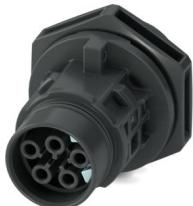
Device connector front mounting, Range of articles: PRC 20, color: black, number of positions: 5, min. conductor cross-section: 0.5 mm<sup>2</sup>, max. conductor cross-section: 2.5 mm<sup>2</sup>, rated voltage: 400 V, rated current: 20 A, Connection method: Screw connection, Setting option for release: 1. with a tool or 2. by hand, scope: SIGNAL
