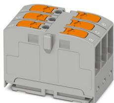
Device terminal block, nom. voltage: 450 V, nominal current: 24 A, number of connections: 6, number of positions: 3, connection method: Push-in connection, cross section: 0.14 mm<sup>2</sup> - 4 mm<sup>2</sup>, Push-in connection, Rated cross section: 2.5 mm<sup>2</sup>, mounting type: for snapping onto a DIN rail adapter, Direct mounting with flange, Free-hanging, color: gray
