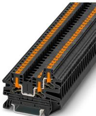
Feed-through terminal block, nom. voltage: 800 V, nominal current: 24 A, number of connections: 3, connection method: Push-in connection, Rated cross section: 2.5 mm<sup>2</sup>, cross section: 0.14 mm<sup>2</sup> - 4 mm<sup>2</sup>, mounting type: NS 35/7,5, NS 35/15, color: black
