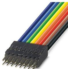
Power connector for DIN rail bus connector with 16 free cable ends with a cross section of 0.25 mm<sup>2</sup>, 500 mm long, male contacts
