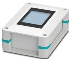
Complete housing for PCBs, can be positioned flexibly, adhesive pads for attaching the PCB, with turquoise blue corner inserts; touch display integrated in housing half-shell, resistive touch technology, 2.4 inch, resolution: 320 x 240 pixels, interface: SPI
