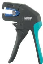
Stripping tool, for cables and conductors (especially for rubber and silicone insulations) from 0.1 - 4 mm<sup>2</sup>, self-adjusting, stripping length of up to 18 mm, cutting capacity of up to 10 mm<sup>2</sup> stranded/1.5 mm<sup>2</sup> solid, replaceable stripping blade
