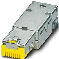
RJ45 male insert, design: RJ45, degree of protection: IP20, number of positions: 8, 10 Gbps, CAT6<sub>A</sub> (IEC 60512-27-100:2008, TIA-568-C.2:2009), material: Metal, connection method: Insulation displacement connection, connection cross section: AWG 26- 24, cable outlet: straight, Ethernet
