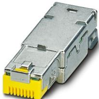
RJ45 male insert, design: RJ45, degree of protection: IP20, number of positions: 8, 10 Gbps, CAT6<sub>A</sub> (IEC 60512-27-100:2008, TIA-568-C.2:2009), material: Metal, connection method: Insulation displacement connection, connection cross section: AWG 23- 22, cable outlet: straight, Ethernet
