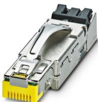
RJ45 connector, design: RJ45, degree of protection: IP20, number of positions: 8, 10 Gbps, CAT6<sub>A</sub>, material: Metal, connection method: Insulation displacement connection, connection cross section: AWG 23- 22, cable outlet: straight, color: yellow, Ethernet
