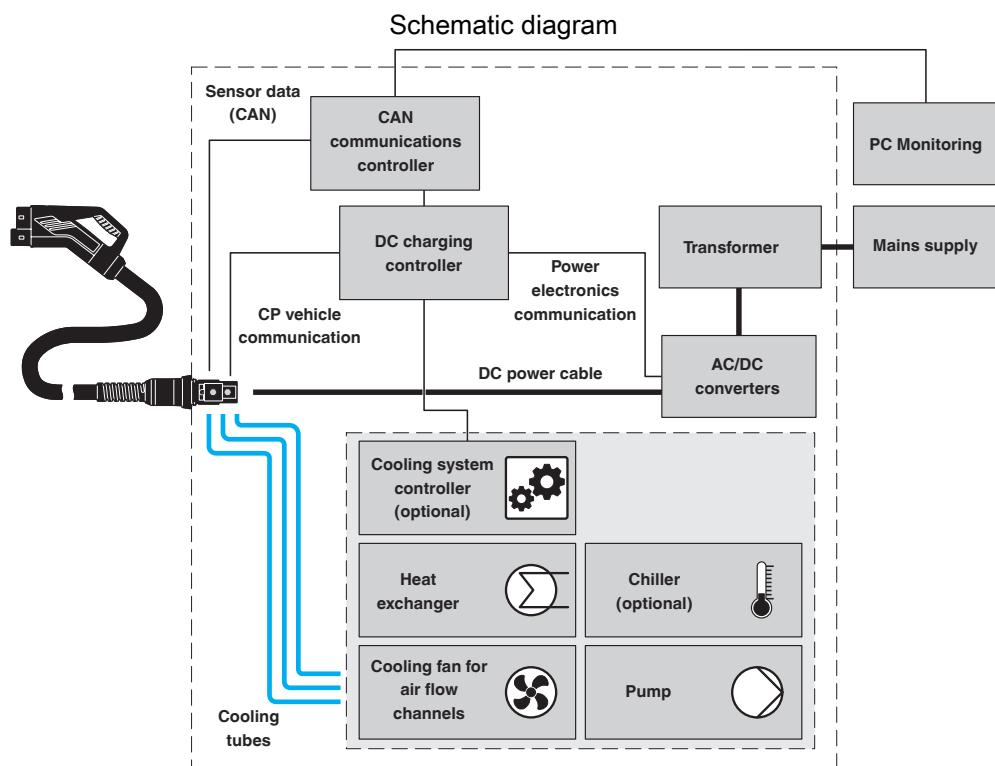
Standalone, decentralized system: cooling unit and controller are integrated into the charging station. The choice of cooling unit can be passive or active (i.e., with or without chiller).
