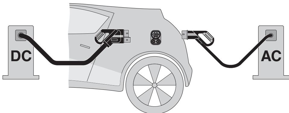
The Combined Charging System (CCS) principle - standard-compliant charging system for electric vehicles, which supports both conventional AC charging and fast DC charging. Both Vehicle Connectors fit into the CCS Vehicle Inlet.
