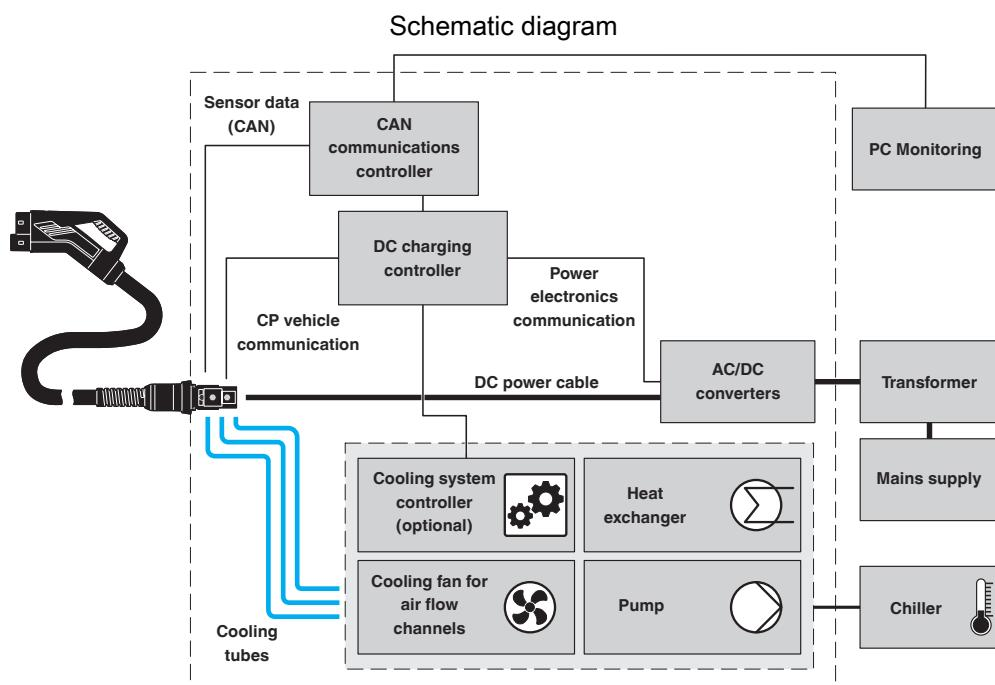
Central system: cooling unit and controller are positioned externally and supply multiple charging stations, each of which is equipped with a heat exchanger. The cooling is done actively using a chiller.
