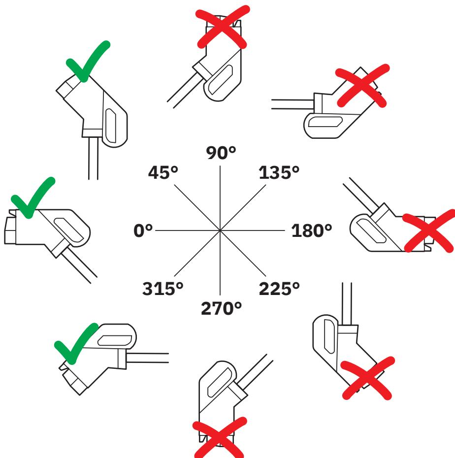
The resting position must be installed in the charging station such that the user cannot hang up the vehicle connector upside down (90° to 270°). However, positions rotated upward (45°) or downward (315°) are options for a resting position.
