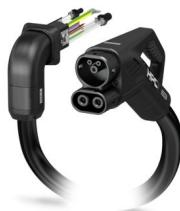
CHARX connect professional, CCS type 2, HPC DC charging cable, 400 A permanent, 1000 V DC, with cooled vehicle charging connector and cooled cable, cable: 5 m, black, straight, with replaceable mating face frame, with replaceable DC power contacts, with right-hand angled panel feed-through, with digital temperature sensors, PHOENIX CONTACT logo, IEC 62196-3-1, for charging electric vehicles (EV) with direct current (DC)
