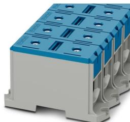
High-current terminal block, nom. voltage: 1000 V, nominal current: 380 A, number of connections: 2, number of positions: 1, connection method: Screw connection, Rated cross section: 240 mm<sup>2</sup>, cross section: 35 mm<sup>2</sup> - 240 mm<sup>2</sup>, Rated cross section: 240 mm<sup>2</sup>, cross section: 35 mm<sup>2</sup> - 240 mm<sup>2</sup>, mounting type: Screw mounting, color: blue
