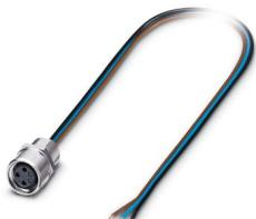
Device connector front mounting, 3-position, Socket, straight, M8, A-coding, Individual wires, cable length: 2 m, 0.25 mm<sup>2</sup>, PVC litz wire
