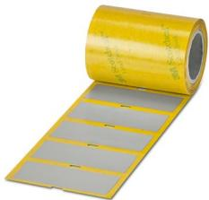
Label, highly flexible, Roll, silver, unmarked, can be labeled with: THERMOMARK E.300 (D)/600 (D), THERMOMARK ROLL 2.0, THERMOMARK ROLL, THERMOMARK ROLL X1, THERMOMARK ROLLMASTER 300/600, THERMOMARK X1.2, mounting type: adhesive, Number of individual labels: 250, text field height: 32 mm, text field width: 85 mm
