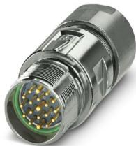
M23, Coupler connector, series: M23 PRO, straight, shielded: yes, for standard and ONECLICK fast locking system, No. of pos.: 16+2+PE, Direction of rotation: Standard, contact connection type: Pin, Crimp connection, cable diameter range: 3 mm ... 15 mm, coding: N, Item is lead-free in accordance with RoHS II without Exemption 6c (Pb < 0.1 %)
