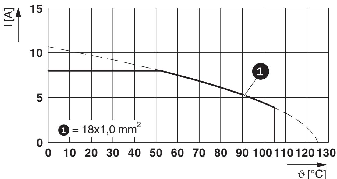
$I$  = current strength,  $\vartheta$  = ambient temperature, 18x 8 A
