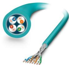
By the meter, Data cable, Ethernet CAT6<sub>A</sub> (10 Gbps), shielded, PUR halogen-free, water blue RAL 5021, 8-wire (4x2xAWG26/7; S/FTP), color single wire: white/blue-blue, white/orange-orange, white/green-green, white/brown-brown, cable length: 300 m
