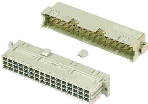
To avoid cross-plugging of adjacent connectors a coding system is required. Insert the code key 09 06 001 9919 into one of the keyways of the female connector as shown in the drawing. Break out the corresponding area of the male shroud. Connectors coded this way can only be applied in a minimum rack spacing of 20.32 mm.
