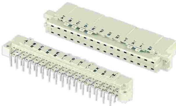
To avoid cross-plugging of adjacent connectors a coding system is required. This coding system is an integral part of both male and female connectors. A comb with 12 coding pins, which is supplied under part number 09 02 000 9928, allows over 900 coding variations. The pins are to be locked into the male and female connectors.
