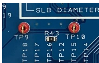
Fig. 4-3-6b Current monitoring resistor and test pins
