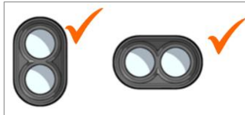
Figure 23: Sensor mounting orientations
