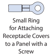
Small Ring for Attaching Receptacle Covers to a Panel with a Screw
