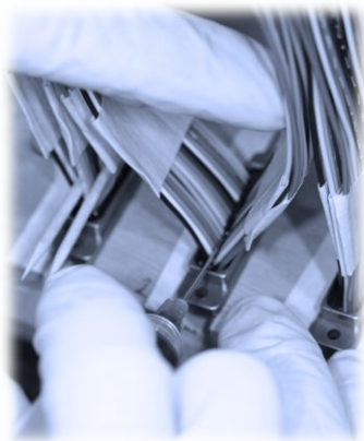
Potting a Micro-D with Epoxy-Filled Syringe
