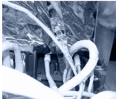
Detail of the Atmospheric Infrared Sounder Instrument (AIRS) with Glenair Micro-D Cables and Connectors
