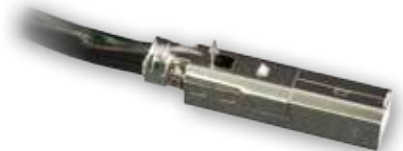
Install insert, attach lid, and crimp shield
