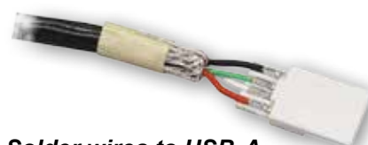
Solder wires to USB-A Insert
