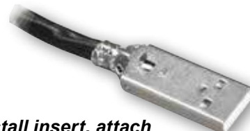
Install insert, attach lid, and crimp shield
