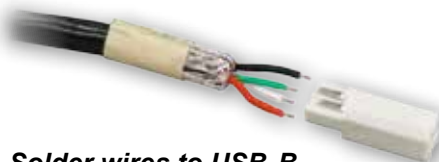
Solder wires to USB-B Insert
