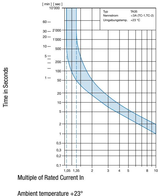
Tripping Characteristics thermal  $I_n \geq 3 \dots \leq 15$  A
